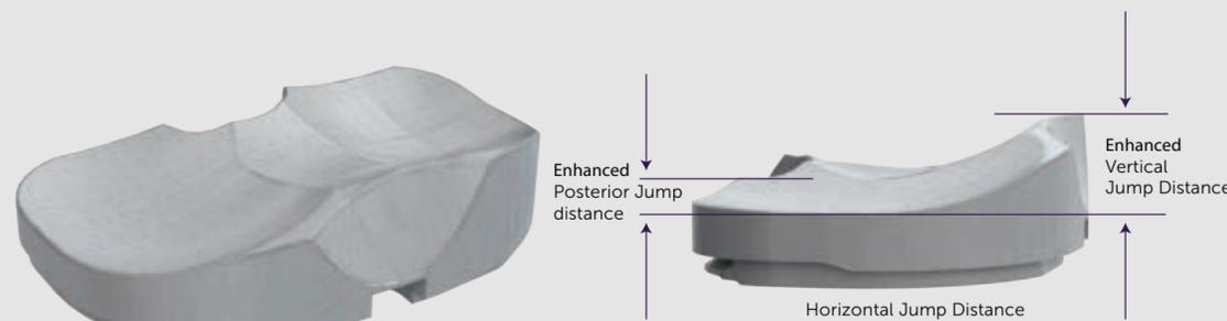
The insert has been designed with deep recess to the patellar groove for patellar tendon relief, the raised anterior medial lip to provide medial stability, with Lateral condyle arcuate path for natural knee function to facilitate rotation of lateral condyle about medial condyle and provide natural knee kinematics. Smooth posterior chamfer of poly insert prevents vital soft tissue impingement.
