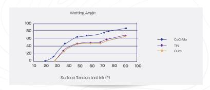
**Higher wettability** means lower contact angle, improved lubrication helps in reduced wear.
