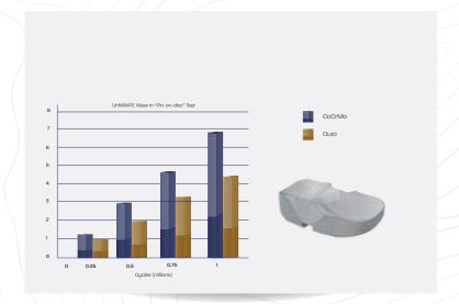
Almost 40% reduction in wear of UHMWPE is observed in a "Pin on disc" test when investigated with 1 million cycles between the uncoated and TiNbN-coated specimens.
